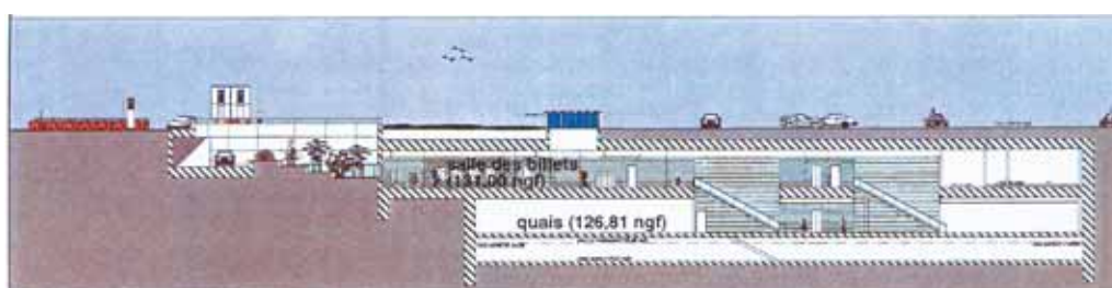
Figure 6 Coupe transversale de la station Balma-Gramont et salle des billets Cross section of Balma-Gramont Station and ticket room
